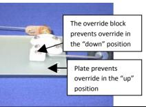
To avoid servo "override", the mounting plate acts as a stop in the up position, and the small block acts as a stop in the down position. The small block will have to be adjusted with sandpaper to fit to obtain the correct angle.
