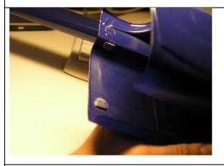
The other pair of magnets should then be glued into the corresponding position inside the nose section.
