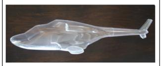
Spot glue the sections together at various points around the fuselage with high viscosity superglue, allow this to set firmly before carrying on with the assembly. When set, run along the seam with a high viscosity superglue to finish off the sealing of the seam
