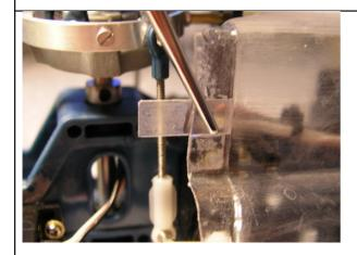
To facilitate the mounting of the nose section, cut some of the scrap Pet-g material to form two small latches either side of the body, as show in the photograph. These are to carry the magnets supplied with the fuselage.
