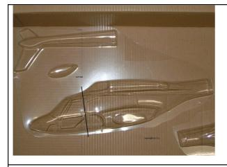
Now the nose section should be separated from the rest of the fuselage. A length of coloured tape placed around the fuselage will act as a guide when cutting. Cut along this line with fine scissors.
