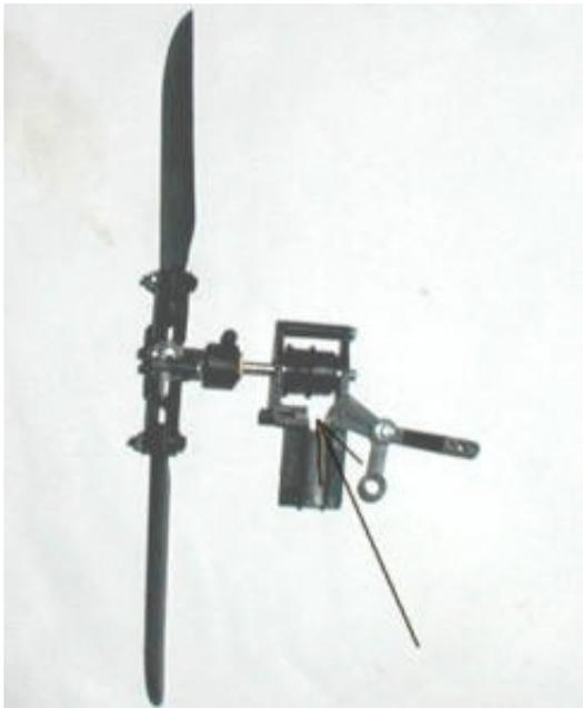
The tail rotor gearbox frame should be cut out at the point shown this will allow for easier assembly of the drive belt.
