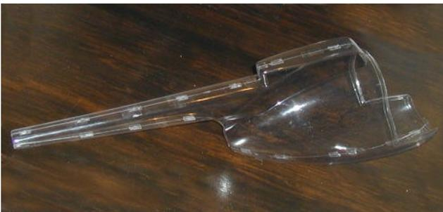
The two halves can now be joined together at regular points using superglue, a rod should be used to exert any pressure required from the inside on each joint. When set, run around the join with thin superglue, and smooth the join with a palette knife.
