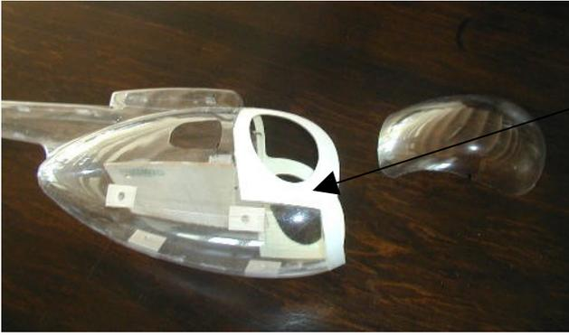
The nose section consists of four separate pieces, a mounting piece, shown in white in the illustration, two side windows and a front window.
