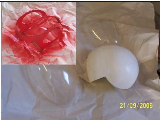
The white nose piece can now be prepared by cutting around where marked. This will produce the nose mounting frame as shown. It can then be spray painted.
