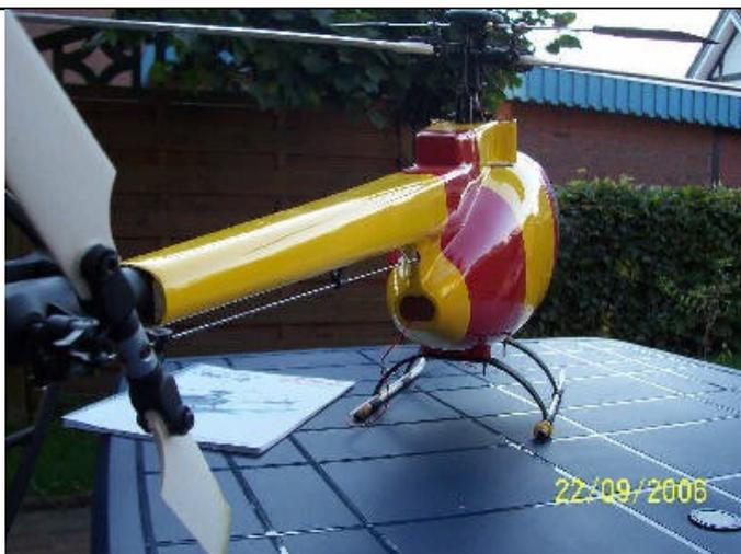
On the Logo 10, the original landing skids are re-used. The skids should be mounted on balsa blocks, these blocks should be glued using plenty of superglue, and reinforced with superglue fillets around the blocks.
