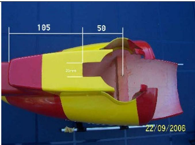
This kit is designed primarily for the ECO 8 therefore some minor modifications are required when fitting to a Logo 10.
