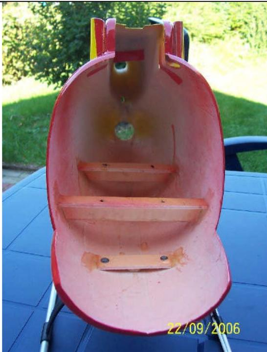
Now the mechanism mounting points are prepared within the fuselage.
