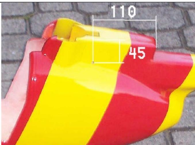
The body should be drilled to accommodate the canopy mounting as used on the original mechanism.
