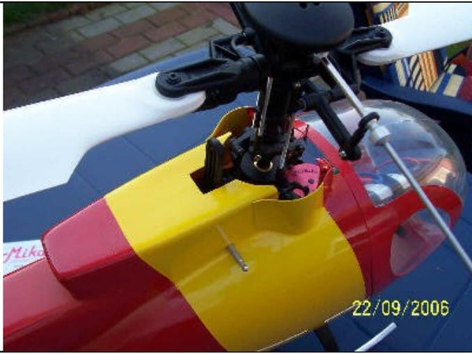
This shows the swashplate mounted, using the original canopy mounting rod.
